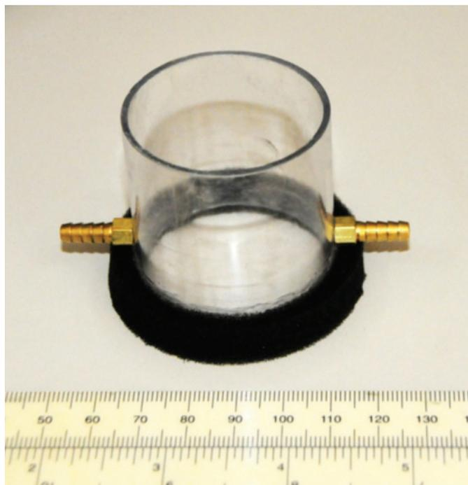
**Figure 3:** Chamber that seals the leaf from the atmosphere, shown here with the lower foam gasket that seals the leaf (sealing material for the objective lens is not shown).
