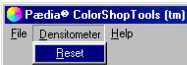
Select "Reset" to reset the densitometer. Do this whenever the densitometer's buttons don't respond. Note: If the densitometer's buttons don't respond, reset it manually: (1) disconnect the densitometer's power cord, (2) wait for the display to go blank. The next time you use it, the densitometer will reset itself.
